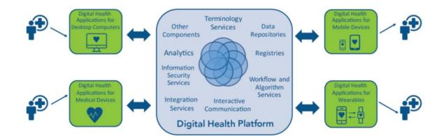
Figure 1: How a DHP interacts with external applications and users.
